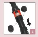
Press firmly on the latch release button and simultaneously pull on the inlet. A slight rotation of the plug may also be required before it can be removed.
