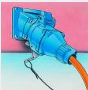
A tension cord is attached to the power cable and the fin pawl of the plug.
