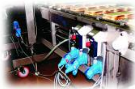
Deconnectors with optional pilot contacts can convey alarms or control auxiliary equipment along a conveyor line.
